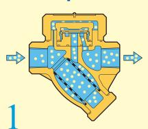
At start-up, the bimetal air vent ring is contracted, lifting the disc off the valve seat and allowing rapid discharge of air and cold condensate.
