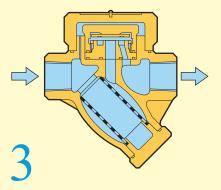
Eventually, the pressure chamber is cooled when condensate enters the space above, lowering the steam pressure in the pressure chamber and thus allowing the inlet pressure to push the disc up and discharge condensate. Entering flashing condensate/steam then closes the trap, as in step 2.
