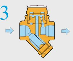
Eventually, as condensate enters the trap and the steam pressure in the pressure chamber lowers, the inlet pressure pushes the disc up and enables the discharge of condensate. Entering flashing condensate/steam then closes the trap, as in step 2.
