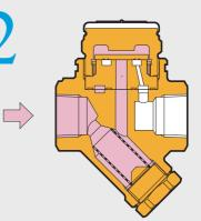
As temperature in the trap rises, the bimetal expands and releases the disc. The disc is forced downward by the low-pressure area created by the rapid flow of flashing condensate/steam below the disc, and the simultaneous high pressure in the pressure chamber above it. An air jacket insulates the cap's pressure chamber from the radiant heat loss that could cause no-load actuation.
