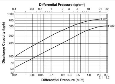
1. Differential pressure is the difference between the inlet and outlet pressure of the trap. 2. Recommended safety factor: at least 2
