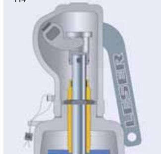
Lift indicator J39: Adaptor for lift indicator H4 J93: Lift indicator
