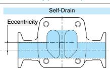
Seat center and straight pipe center are eccentrically positioned and the bottom end of valve seat is in line with inner wall of straight pipe.
