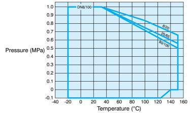
\* Lower limit temperature for PFA lined main body made of base material FCD-S is -10°C
