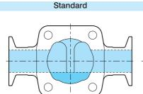
The valve seat is on the same centerline with straight pipe.
